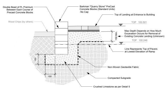
Pre-Cast Concrete Block Wall & Paving at Top of Landing - Barkman Quarry Stone
